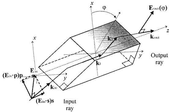
Fig. 1. Arbitrary propagation of polarized light through a simple rotational prism (Dove prism). The ray path is given by unit vectors  $\mathbf{k}_{in}$ ,  $\mathbf{k}_1$ ,  $\mathbf{k}_2$ , and  $\mathbf{k}_{out}$ .
